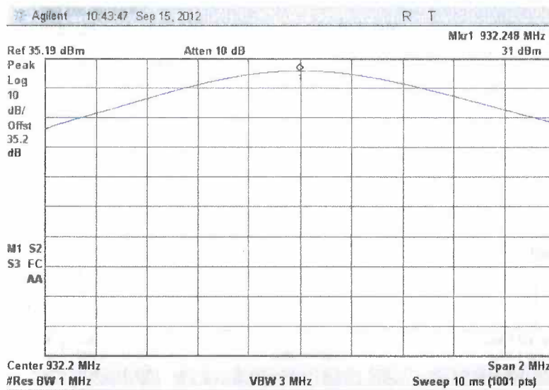
Figure 7.1.2-5: Peak Output Power 932.25 MHz
